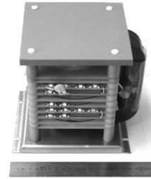
Fig. 4: The high voltage transformer assembly.
